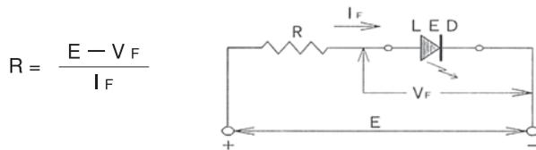
Current to be applied on LED must be lower than the forward current ( $I_F$ ) indicated in the LED specification column of each switch. Value of the resistor must be calculated by the formula noted below.
